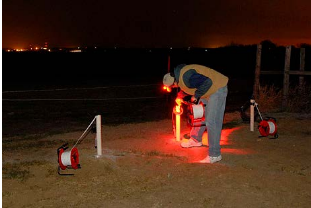
A United States Geological Survey researcher measures groundwater levels in a well near Oakland, Nebraska. (Photograph courtesy USGS Multimedia Gallery.)
