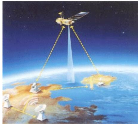
**Image to left:** SLR Supports Sensing of Surface Elevations: Satellite Laser Ranging (SLR) provides direct, clear measurements of surface heights of sea level and land surfaces, using satellites and SLR stations on the ground that cross-check each other. Accurate SLR measurements provide changes in the global mean sea level to a few millimeters per year. Credit: NASA
