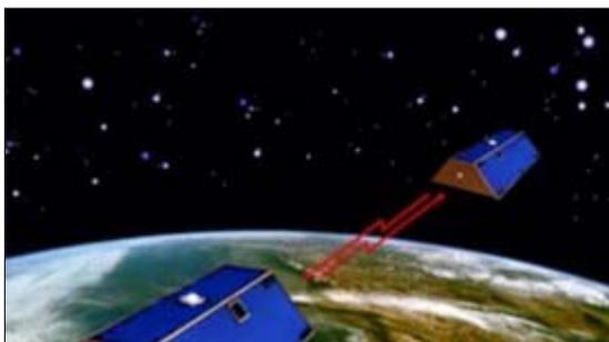
**Left:** The twin GRACE satellites will use hyper-sensitive microwave range finders to measure the distance between them. Image courtesy [NASA's Jet Propulsion Laboratory](#) .
