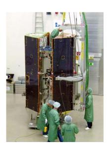
The GRACE satellites were developed and manufactured for NASA/JPL by Astrium GmbH in Friedrichshafen and tested at IABG in Ottobrunn. (Fig: Astrium)
