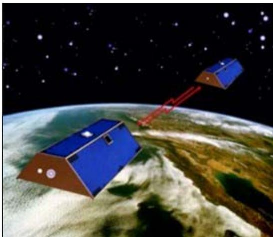
**Left:** The twin GRACE satellites will use hyper-sensitive microwave range finders to measure the distance between them. Image courtesy [NASA's Jet Propulsion Laboratory](#) .
