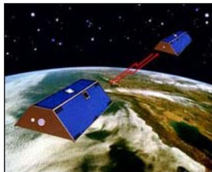
A drawing of the twin GRACE satellites. The satellites will use a microwave beam, depicted here by the red lines, to keep track of each other
